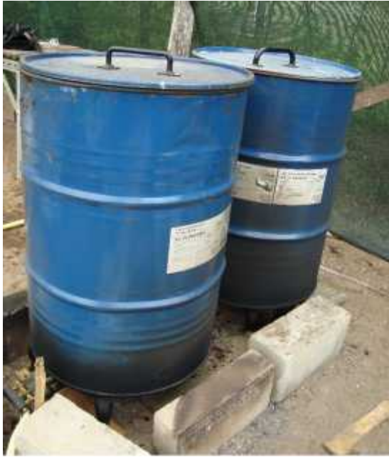
Figure 15. Self-made soil steamer with barrels during experiment at AdeKUS Leysweg
